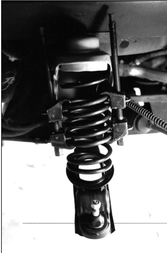
Compressed spring ready for removal.
